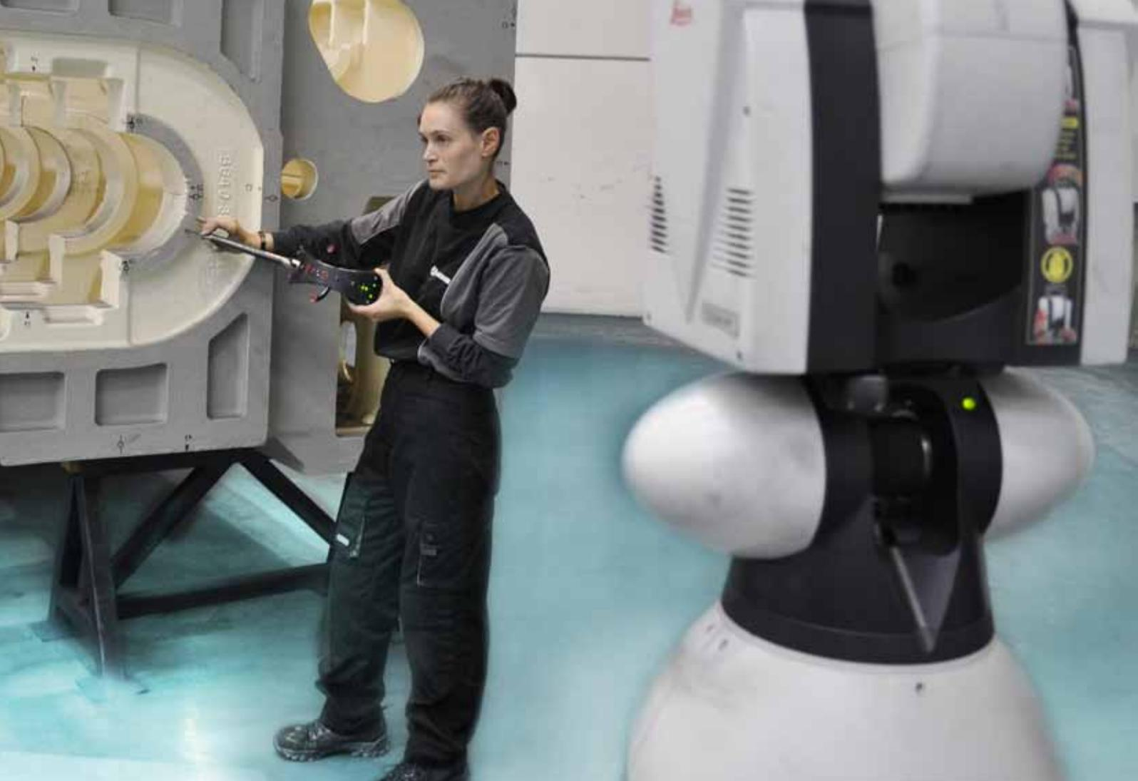
*Inspection of an engine block*
