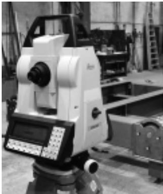
Leica TDM5005 with integrated DCP05 software
