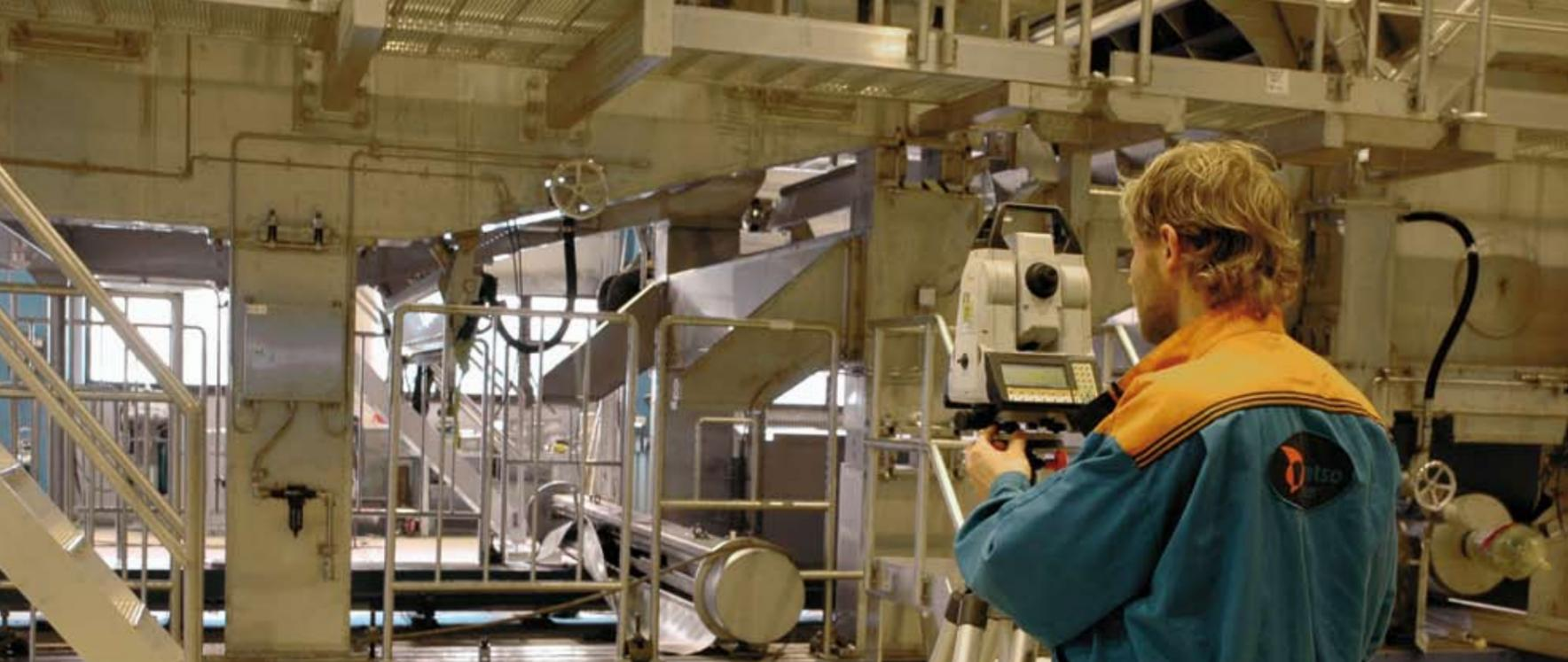
Setting up the Leica Geosystems Total Station takes up a mere 2 minutes, whereas the previous systems consisting of a theodolite and a level took about 10 minutes to set up. The time savings amass exponentially because one Total Station setup can cover several measurement points, while a theodolite-based system needs to be set up anew for each new point being inspected.
