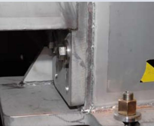
Despite their massive weight and size, these cantilever beams at the base of the machine need to be brought into position with accuracies of 0.1mm.
