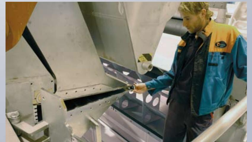
The position of the insertion axis and its parallelism to the rollers is checked with a reflector. The Total Stations can automatically locate the reflector, significantly shortening the inspection times and removing the human error factor from the equation.
