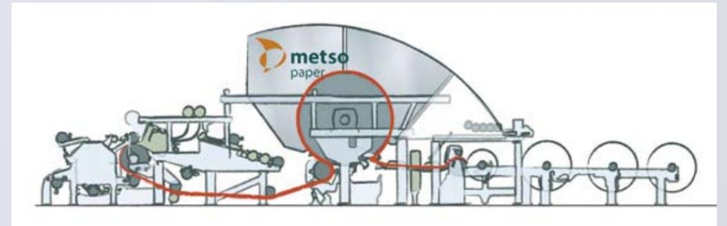
A typical paper line machine may have in excess of 20 rolls needing alignment. Anywhere between 20 and 40 meters in length, it may weigh more than 250 tons. The red line traces the paper path in the machine.
