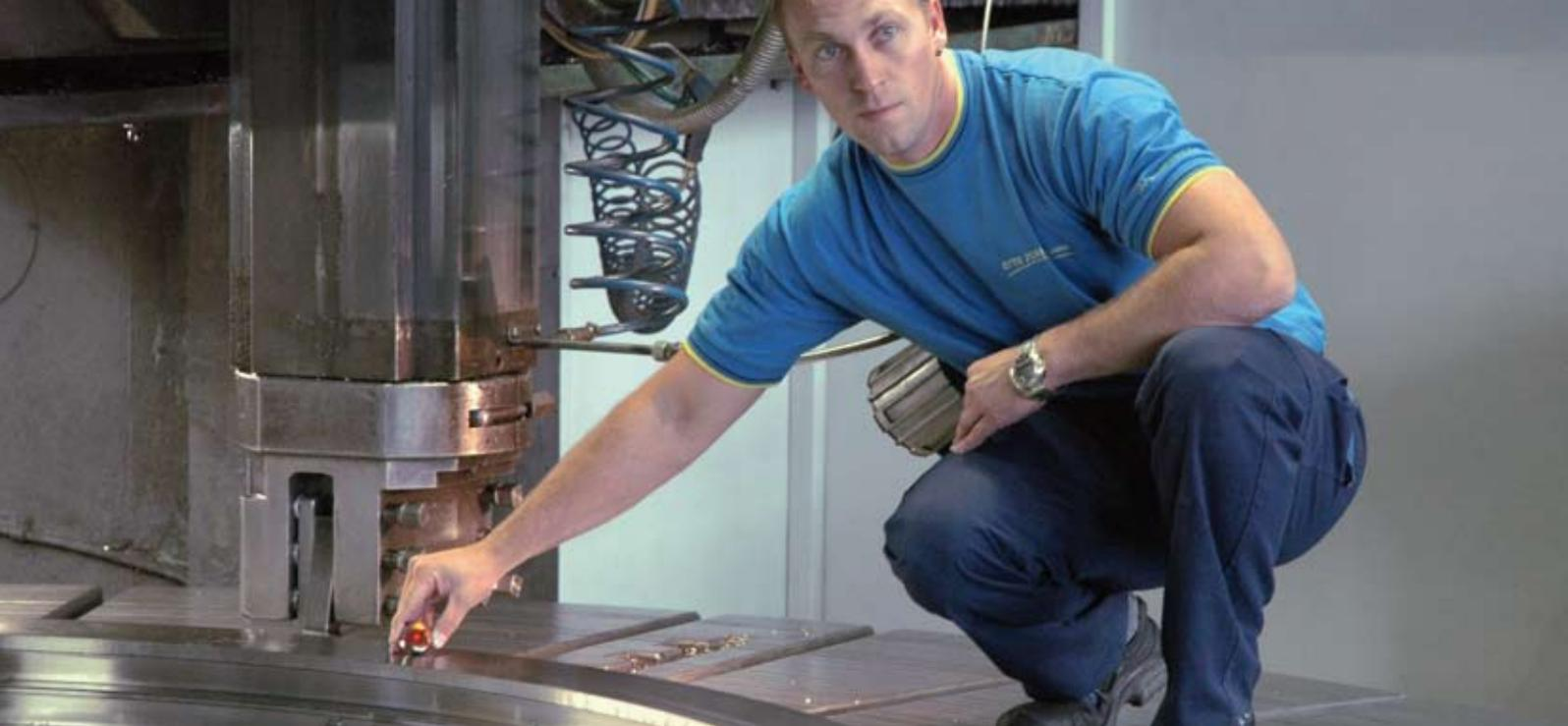
Measuring directly on the turning mill: Michael Gerards, Precision Mechanics Foreman, checks about 30 points on the casting using a reflector
